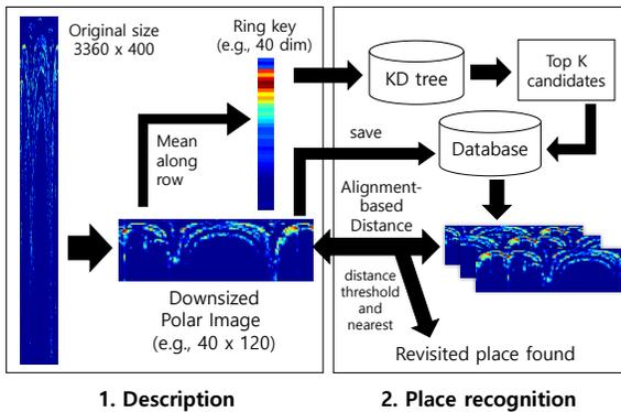
Fig. 8: A pipeline of Scan Context-based [2] radar place recognition method. We use the jet color map for visualization clarity; we use the intensity polar image directly, only downsampling with pixel interpolation.
