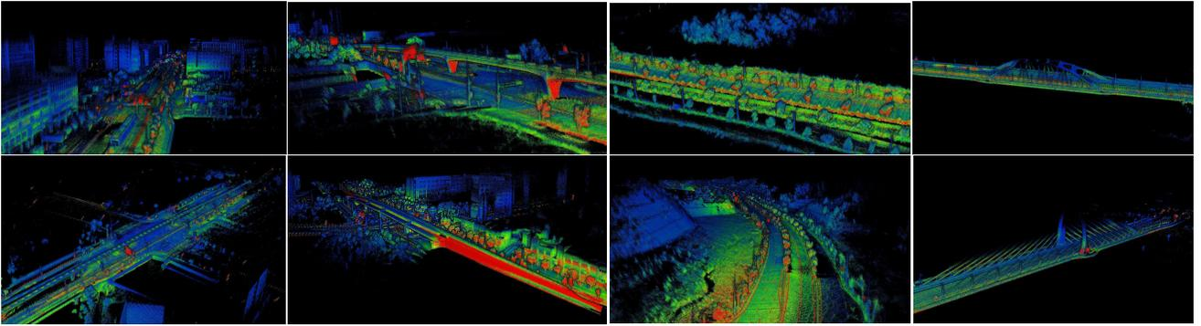
Fig. 6: Structural diversity in a single sequence (*Sejong 01*). These captures are taken from a point cloud map using our 3D LiDAR. The color map represents an intensity value of each point (red is high).
