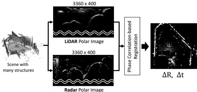
Fig. 3: Extrinsic calibration between the LiDAR and the radar using phase correlation [33].
