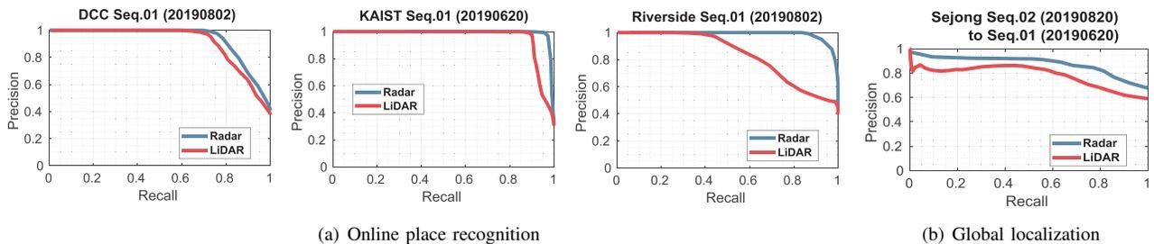
Fig. 9: Radar outperforms LiDAR for urban place recognition.
