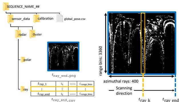
(a) The data structure of a sequence (b) Information within radar data
