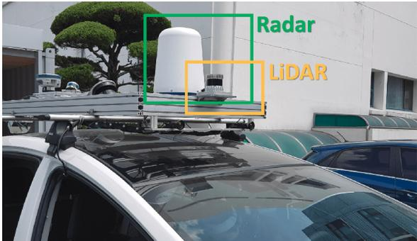
Fig. 2: The sensor system is equipped with a single radar and a 3D LiDAR sensor, providing multimodal range measurements.
