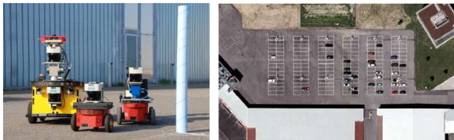
Figure 7.8: Three robots and a synthetic landmark used in the multi-robot mapping experiment from [35] (left), and an aerial view of the parking lot in which the experiment was performed (right).
